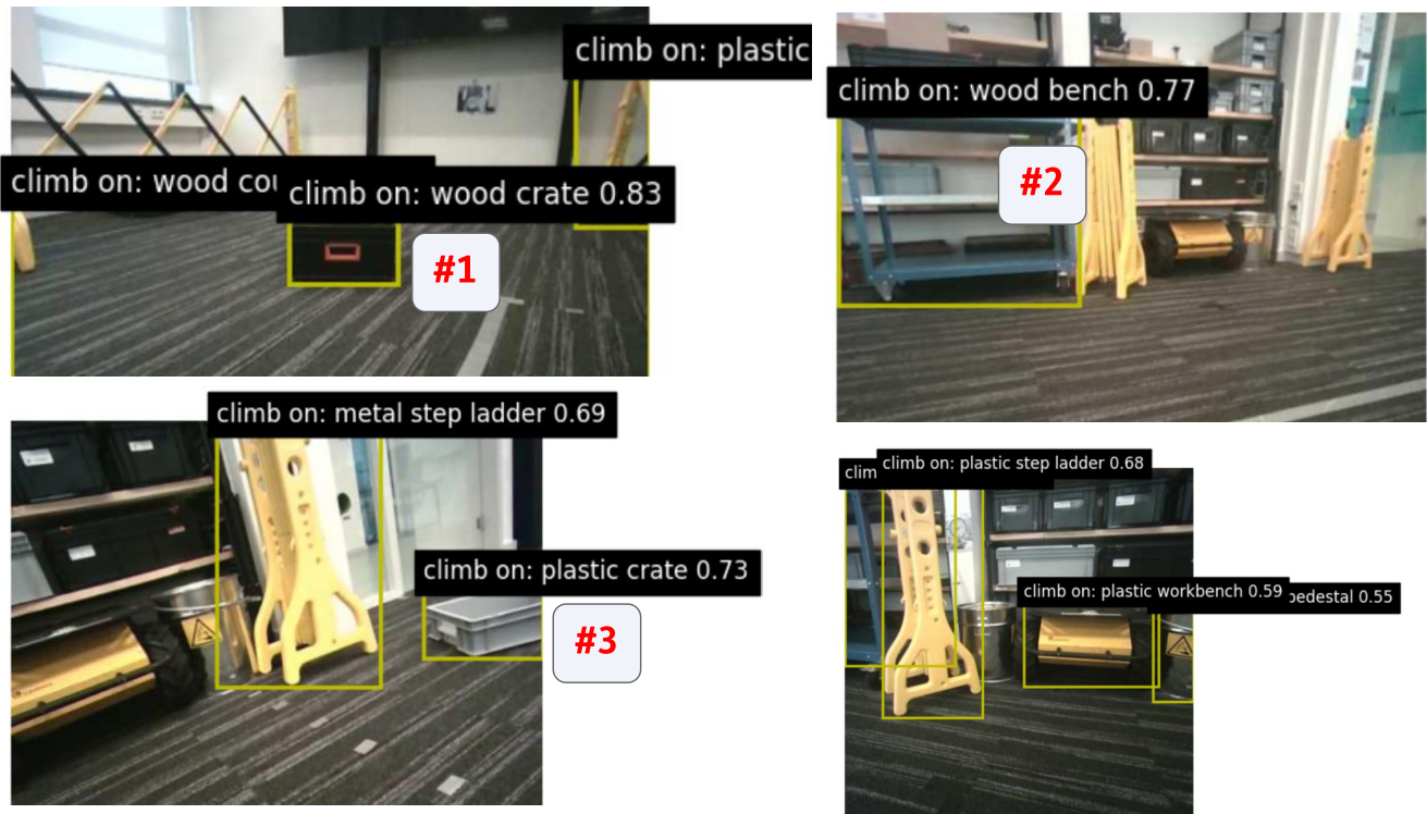
Fig. 8: Robot: With our method, the robot finds a Wooden Crate (top left) when the intended action is ‘climb on’.
